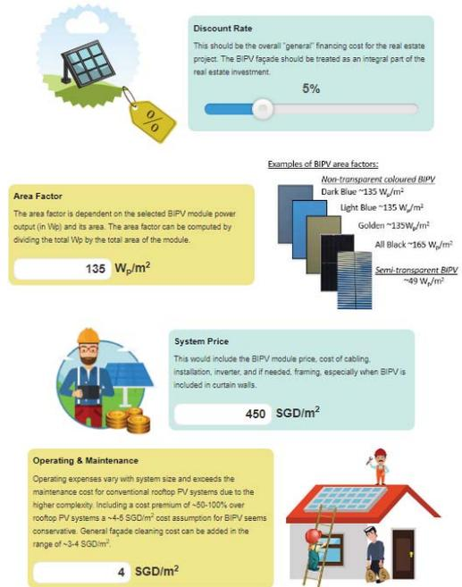
Figure 4. Details of the BIPV system, economics and efficiency factors in online toolkit.
