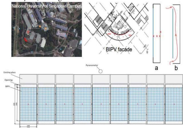
Figure 1. Location and technical details of the a – non-ventilated BIPV façade, and b- ventilated BIPV facade at the School of Design and Environment, NUS.
