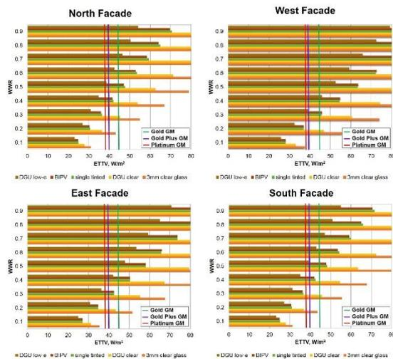
**Figure 5:** ETTV sensitivity analysis when changing the thermal properties of the glazing (SHGC) and the window-to-wall ratio (from 0.4 as best case to 0.9 fully glazed facade). The Gold and Gold Plus and Platinum Green Mark Award requirement are marked with green, purple and red lines, respectively.
