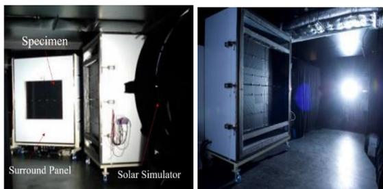
**Figure 2:** Photographs of the metering box with installed specimen (left), and indoor sun simulator (right).
