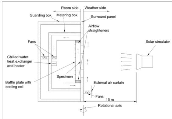
**Figure 1:** Schematic drawing of the experimental set-up of SERIS' Calorimeter Hot Box for Solar Heat Gain Coefficient (SHGC) measurements.
