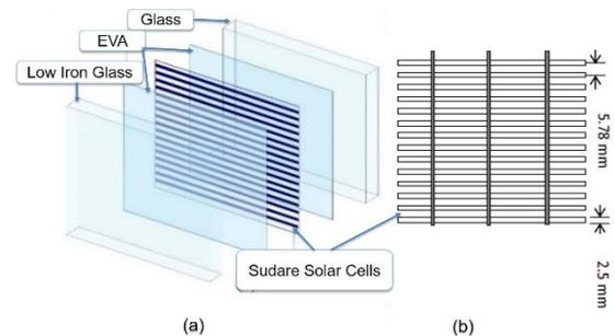
**Figure 4:** Multifunctional glazing element: (a) glass-glass BIPV layers configuration; (b) detailed design of cell arrangement.
